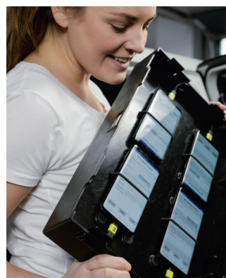
Each drive test vehicle carried nine smartphones for the voice and data tests.
