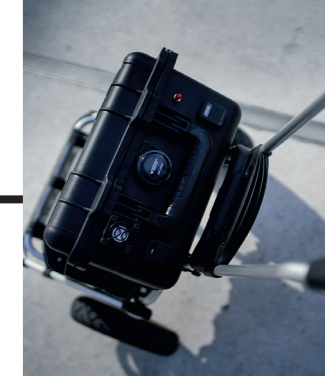
The walktest teams use trolleys or backpacks in which powerful batteries feed the test smartphones.
