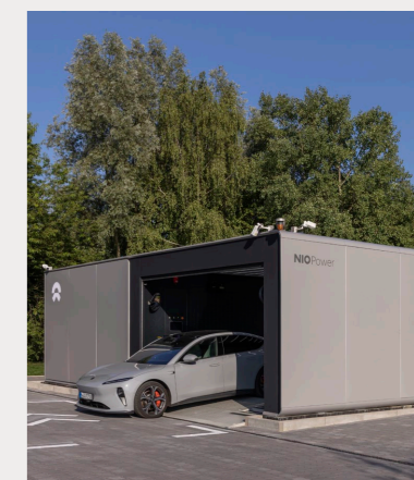
Innovative: In the "Power Swap Stations", an ET7 is implanted with a fully charged battery within five minutes.
