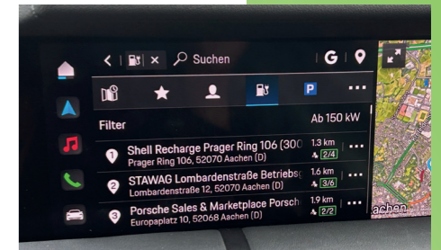
Dependent: A charging strategy that takes into account the availability of charging points needs reliable real-time data from the stations on site.
