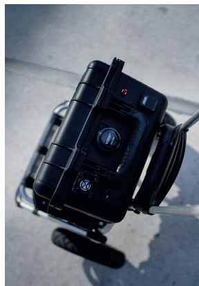
The walktest teams use trolleys in which powerful rechargeable batteries feed the test smartphones.
