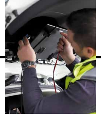
Boxes mounted to the rear and side windows of the cars contain the smartphones used for testing.
