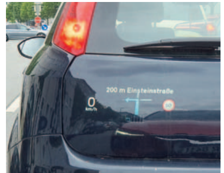
The navigation view of the optional head up displays is great. It makes turning the driver's eyes to the cockpit or central display obsolete.
