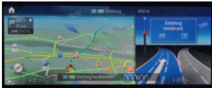
3D maps and maneuver info in split screen style as well as lane recommendations are displayed in a well-arranged manner.
