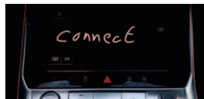
The climate control display not only accomodates the user's shortcuts, but also serves as an input area for text, depending on the current functions.
