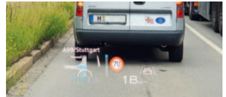
The e-tron's head up display offers a very precise representation of the next maneuver including an accurate lane recommendation.
