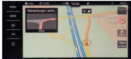
In addition to the lane recommendations in the upper area, the system also presents turn indications including traffic signs.
