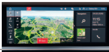
A swipe to the left invokes the split screen view. From there, swiping up or down accesses the following contents.
