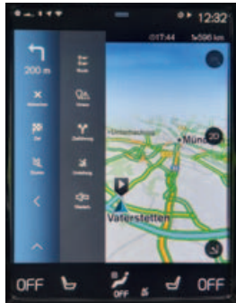
The two columns on the left-hand side of the screen contain the navigation options. The 3D view shows an unnecessarily large amount of sky.
