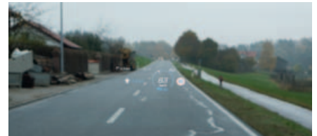
The headup display is offered at a surcharge, but gives reliable information about speed, traffic signs and navigation maneuvers.
