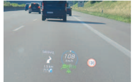
The clearly readable presentation of navigation instructions in the head up display impressed the testers.
